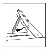
To use the wheel blocks, lift the wheel block as shown and lock into place. Then, use the following as a guide to assist you in the placement of the wheel blocks.
